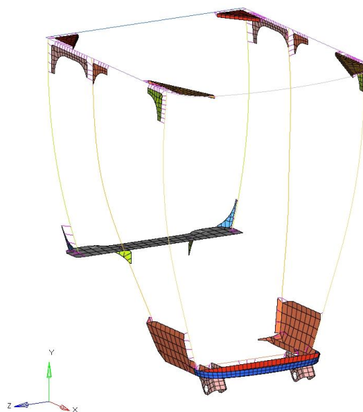
Fig 2. Finite Element Model of ROPS – 1D Beam, Bar & Spot – Weld Elements
